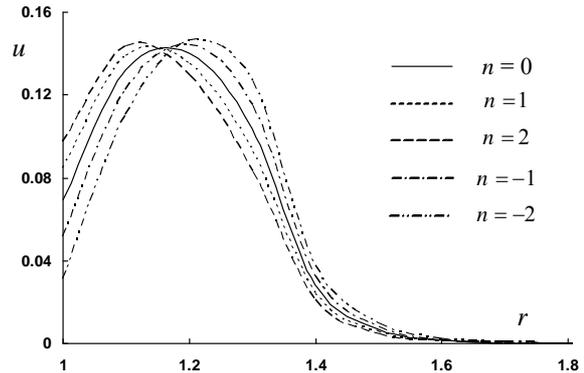
**Figure 1.** Variation of displacement with respect to radius for different values of nonhomogeneity parameter  $n$ .
