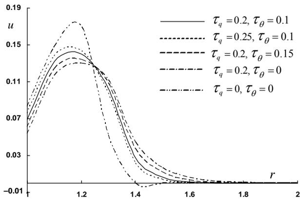
Figure 5. Variation of displacement with respect to radius for different values of phase-lags.
