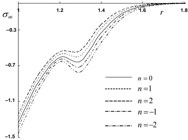
Figure 4. Variation of hoop stress with respect to radius for different values of nonhomogeneity parameter  $n$ .
