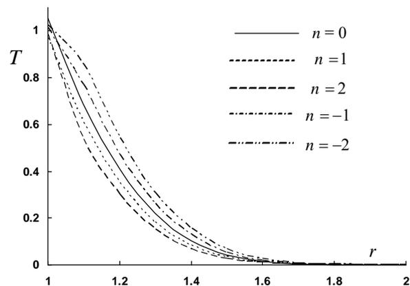
**Figure 2.** Variation of temperature with respect to radius for different values of nonhomogeneity parameter  $n$ .
