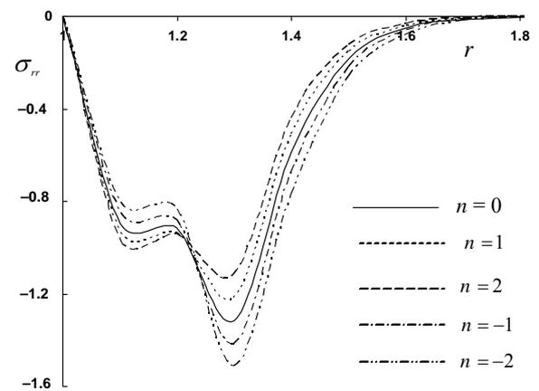
**Figure 3.** Variation of radial stress with respect to radius for different values of nonhomogeneity parameter  $n$ .
