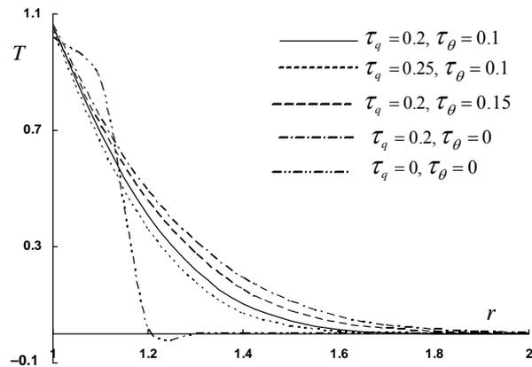
Figure 6. Variation of temperature with respect to radius for different values of phase-lags.
