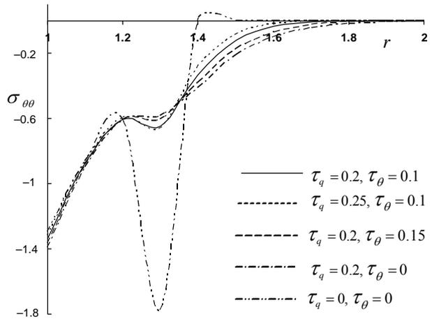
Figure 8. Variation of hoop stress with respect to radius for different values of phase-lags.
