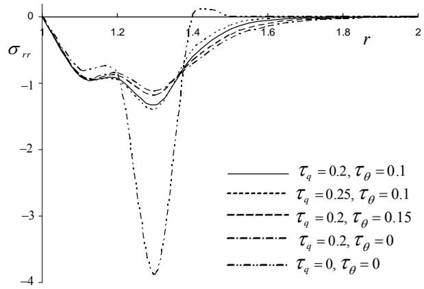
Figure 7. Variation of radial stress with respect to radius for different values of phase-lags.
