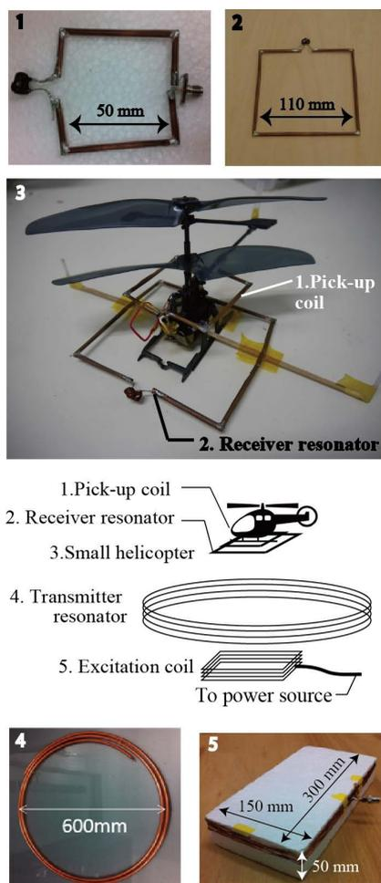
**Figure 1.** Wireless power transfer system for the small helicopter.
