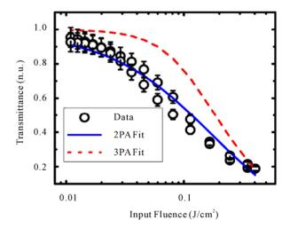
Figure 4. Optical limiting cure recorded for PC3 in PMMA. Blue (solid) line is the fit for 2PA while red (dotted) line is the fit for 3PA.
