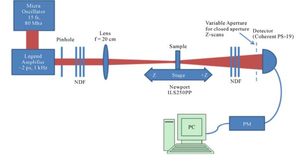
Figure 1. Experimental set up used for open aperture and closed aperture Z-scans. NDF stands for neutral density filters and PM stands for power meter.
