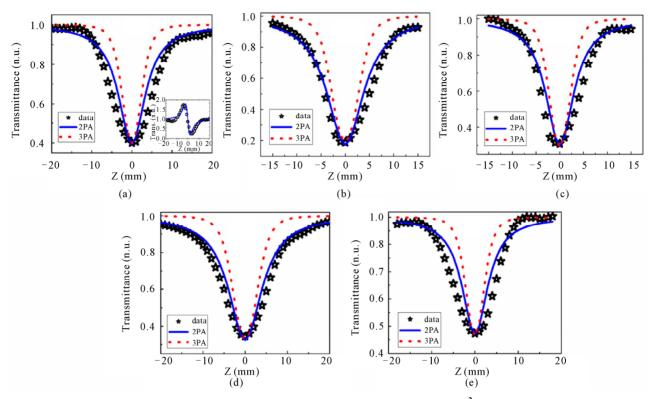
Figure 3. OA Z-scan curves of PC1 to PC5 recorded with peak intensity of 200 GW/cm<sup>2</sup>. Open stars represent the experimental data while the solid lines are fits. Red (dotted) and blue (solid) lines represent theoretical fit for 3PA and 2PA, respectively. Inset of (a) shows CA scan recoded at same intensities.
