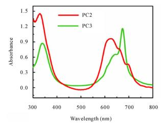
Figure 2. UV-visible absorption spectra of PC2 (top, red color) and PC3 (bottom, green color) doped in PMMA.
