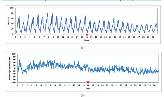
Figure 4. (a) The daily TEC variation for the month of April 2013 obtained at Surat station; (b) Percentage deviation in TEC from monthly mean for Surat Station. Star indicates the Earthquake day.
