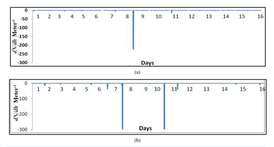
**Figure 5.** (a) The radio refractive index gradient dN/dh for Shiraz, Iran. It is seen that the dN/dh reduced beyond the critical limit  $\langle -157 \text{ Km}^{-1} \text{ on } 8 \text{ April 2013}$ ; (b) The radio refractive index gradient dN/dh for New Delhi. It is seen that the dN/dh reduced beyond the critical limit  $\langle -157 \text{ Km}^{-1} \text{ on } 8 \text{ and } 11 \text{ April 2013}$ .
