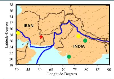
Figure 1. Show the Map of the faultline (blue line) of the Iran earthquake. The red star indicates the epicenter and the yellow and green circles show the radiosonde and GPS stations. Both the radiosonde stations are very close to the faultline and so can be the best choice to study the atmosphere around the faultline prior to an earthquake.
