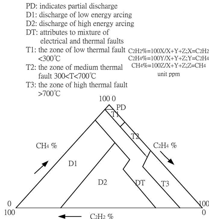
**Figure 2.** IEC-Duval triangle method [3].
