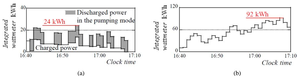
**Figure 5.** Capacity in the electric accumulator. (a) With power stabilization system; (b) Without power stabilization system.
