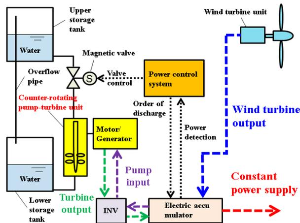
**Figure 1.** Power stabilization system.
