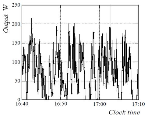
**Figure 2.** Output from the wind power unit in house.
