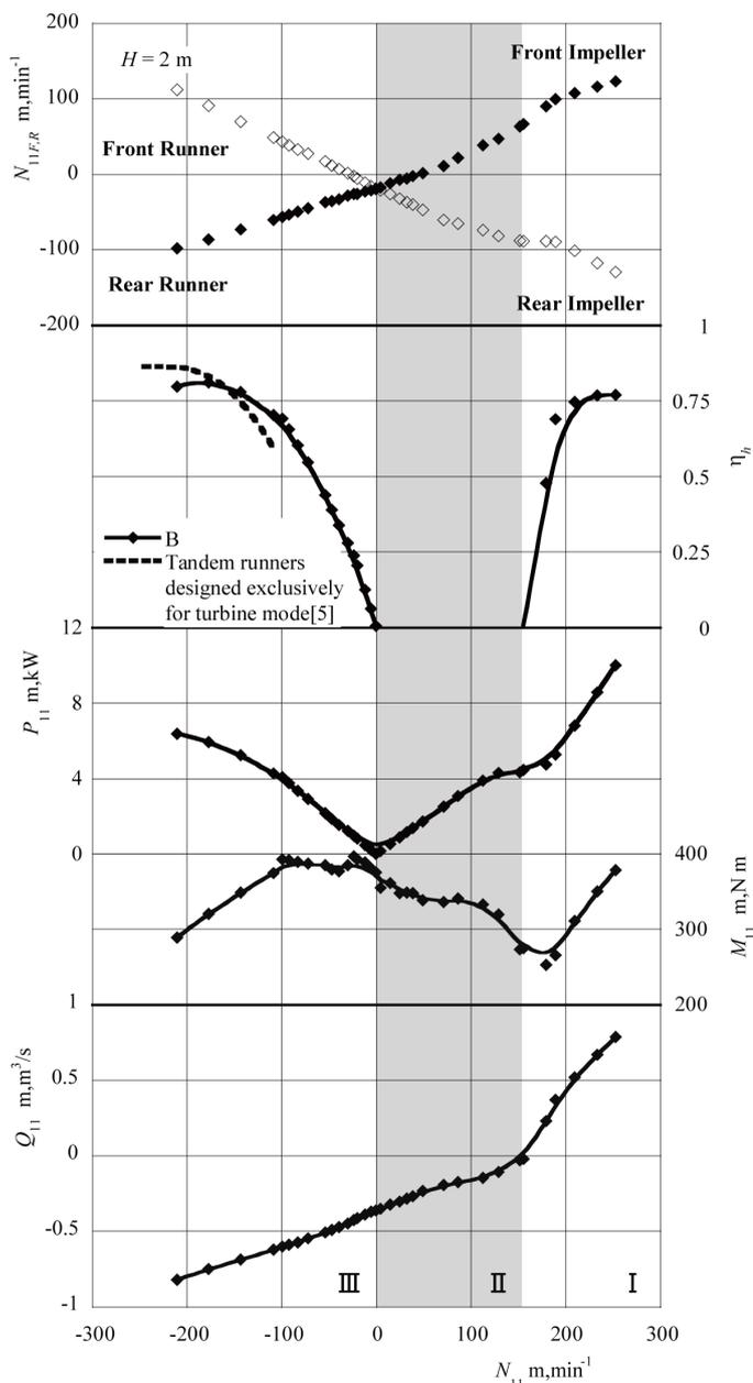
**Figure 8.** Overall performances of the counter-rotating type pump-turbine unit.
