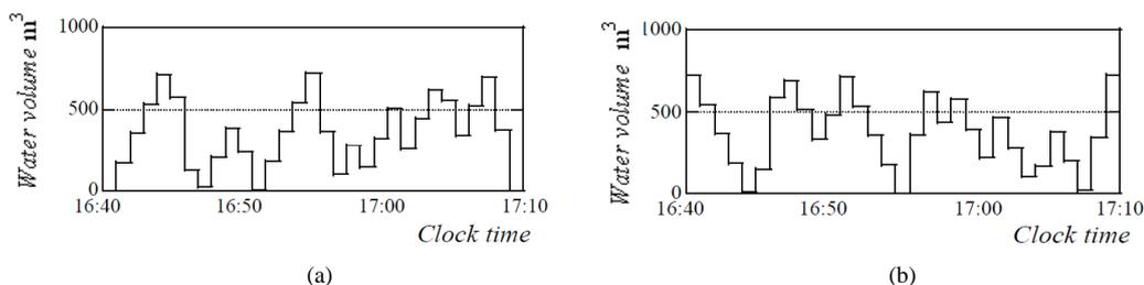
**Figure 4.** Water volume in the storage tanks. (a) Upper storage tank; (b) Lower storage tank.
