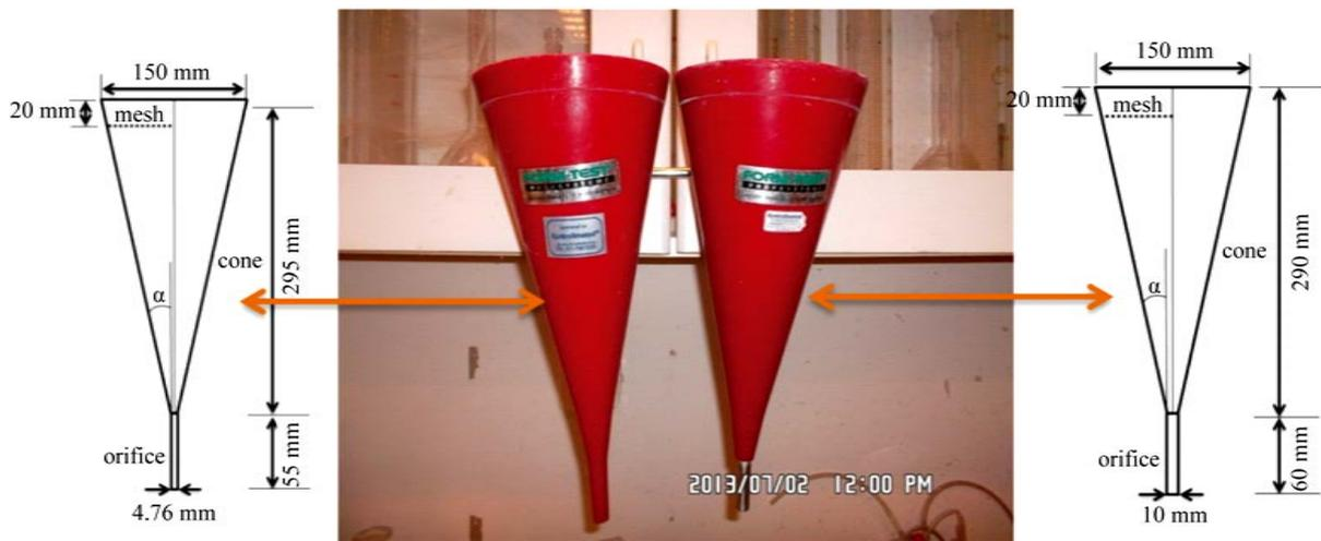
Figure 7. Marsh funnel, left: small one (4.76 mm orifice), right: the big one (10 mm orifice).
