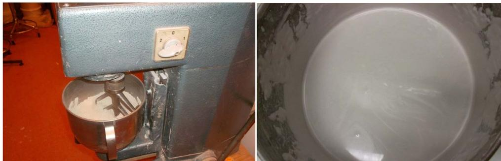
**Figure 5.** Grout mixture preparations with the degree of fluidity being illustrated by the right figure.
