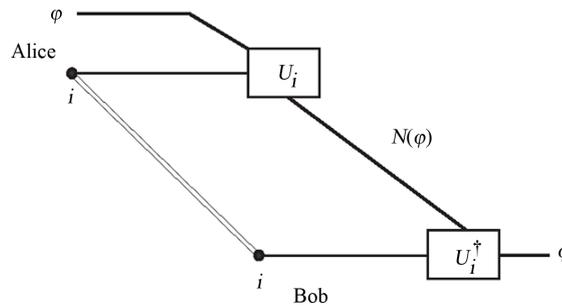
**Figure 1.** Private quantum channel: Alice applies  $U_i$ 's for encoding of  $\varphi$  and Bob decodes  $N(\varphi)$  with a secret key  $i$  which is pre-shared  $\log n$ -bits of classical information.
