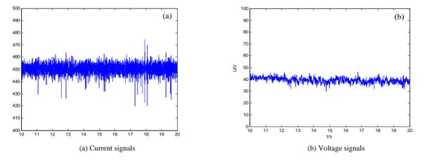
Figure 3. The arc signals under experimental program (c).
