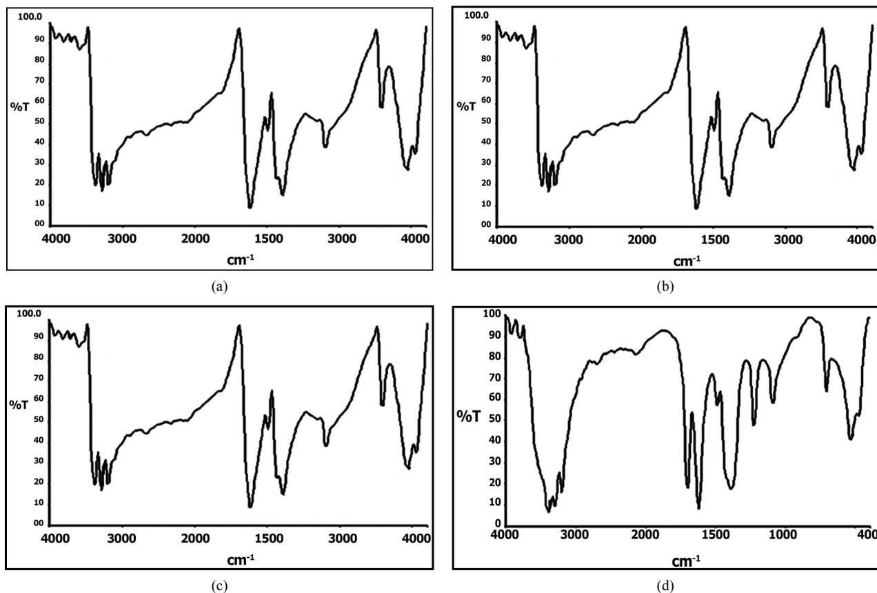
**Figure 3.** (a) FTIR Spectrum of BTCC; (b) FTIR Spectrum of 1 mole %, ZnCl<sub>2</sub> mixed BTCC; (c) FTIR Spectrum of 5 mole % ZnCl<sub>2</sub> mixed BTCC; (d): FTIR Spectrum of 10 mole %, ZnCl<sub>2</sub> mixed BTCC.
