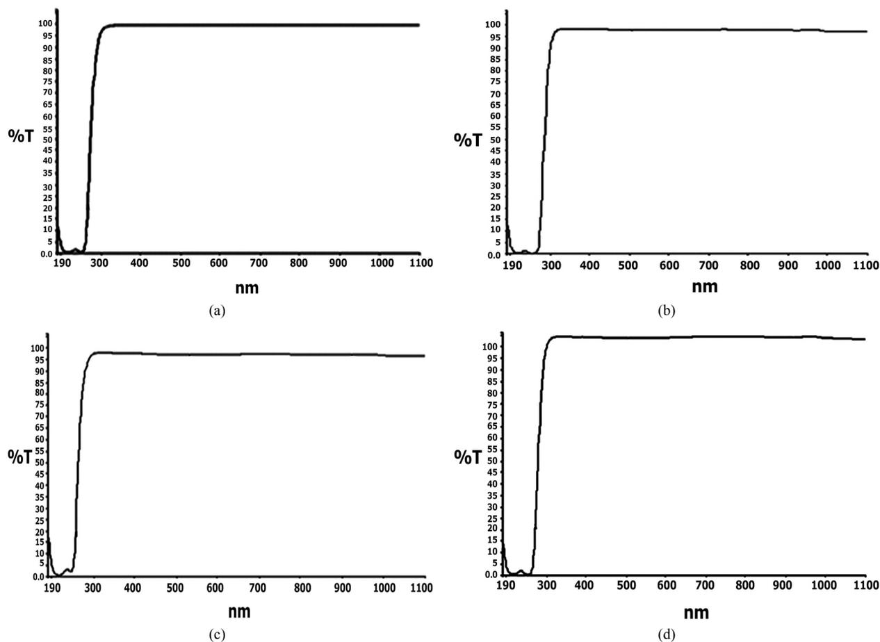
Figure 4. (a) UV-Vis-NIR spectrum of BTCC; (b) UV-Vis-NIR spectrum of 1 mole %  $ZnCl_2$  mixed BTCC; (c) UV-Vis-NIR spectrum of 5 mole %  $ZnCl_2$  mixed BTCC; (d) UV-Vis-NIR spectrum of 10 mole %  $ZnCl_2$  mixed BTCC.
