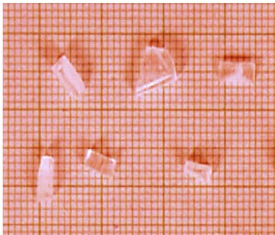
Figure 1. Photograph of pure BTCC Crystals.
