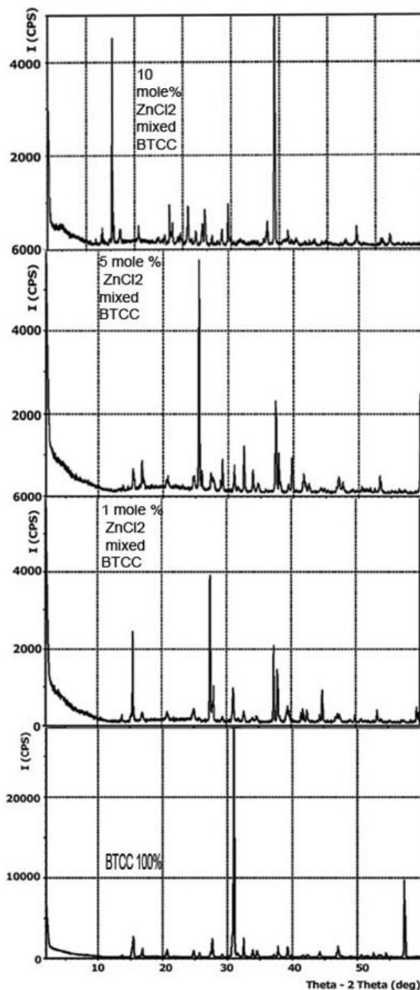
Figure 2. Powder XRD pattern of BTCC and  $\text{ZnCl}_2$  mixed BTCC.
