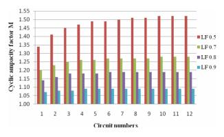
Figure 3. Relationship between cyclic ampacity factor M and circuit numbers.
