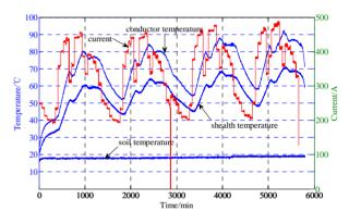
Figure 2. Graph of LF 0.7 single-loop direct buried cable cyclic ampacity experiment.
