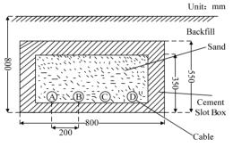
(b) The sectional view of laying of the experimental cables
