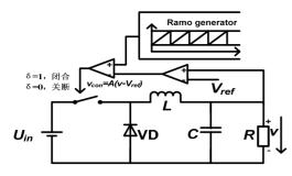
Figure 2 .Voltage type Buck converter.
