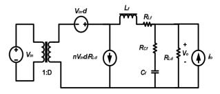
Figure 3. Buck converter small signal model.
