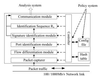
Figure 2. Extensible P2P flow identification architecture.
