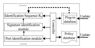
Figure 4. Online updating mechanism of EPFIA.
