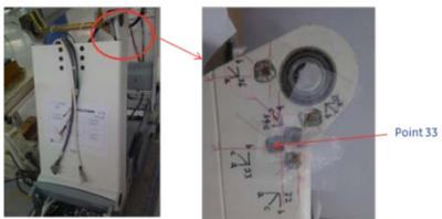
Figure 5. Measurement points on front leg.
