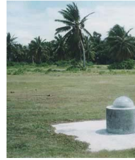
Fig. 8 COCO station is equipped with an ASHTECH UZ-12 GPS receiver with an AOAD/M T antenna type. This station is located within the perimeter of Cocos Island Airport and it offers unobstructed visibility of the sky (Geoscience Australia, 2007).
