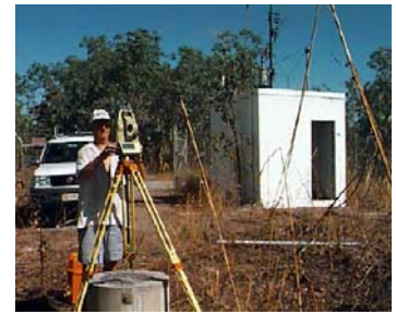
Fig. 9 DARW station is equipped with an ASHTECH UZ-12 GPS receiver with an ASH700936D_M antenna type. This station is located at an old abandoned seismic station at Manton Dam and is surrounded by trees and a building (Geoscience Australia, 2007).
