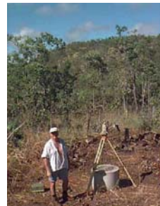
Fig. 9 DARW station is equipped with an ASHTECH UZ-12 GPS receiver with an ASH700936D_M antenna type. This station is located at an old abandoned seismic station at Manton Dam and is surrounded by trees and a building (Geoscience Australia, 2007).
