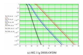
Figure 3. Frame error rate of IEEE 802.11a/g fixed LAN over Rayleigh fading channel.
