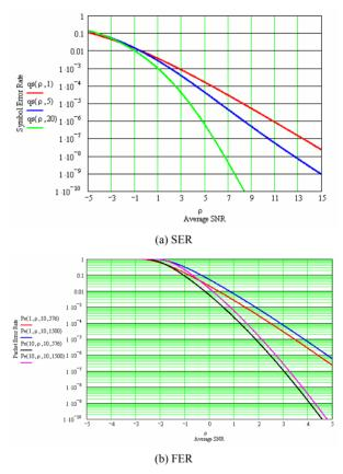
Figure 4. SER and FER of IEEE 802.11n fixed LAN over Rician fading channel.
