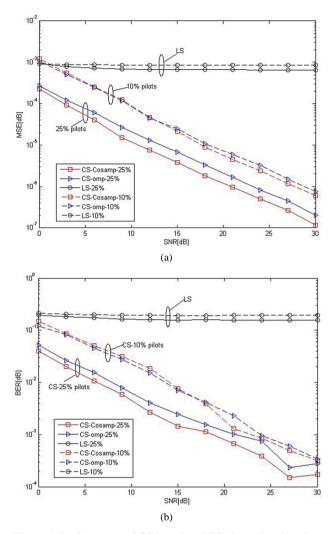
Figure 1. Performance of CS-based and LS channel estimation. (a): MSE versus SNR; (b): BER versus SNR.
