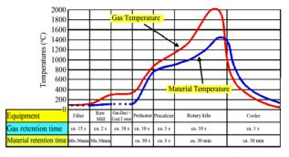
Figure 2. High-temperature calcination of rotary kiln.
