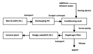
Figure 6. Flow sheet of deep dewatering.
