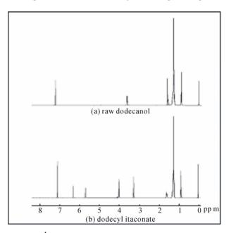
Figure 2. <sup>1</sup>H NMR spectra of (a) raw 1-dodecanol, (b) synthesized dodecyl itaconate. (in solvent CDCl<sub>3</sub>).
