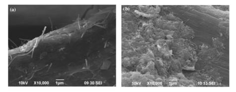
Figure 4. SEM micrographs of dispersed CNTs on single cellulose fiber (a) in the acid and (b) in the general papermaking.
