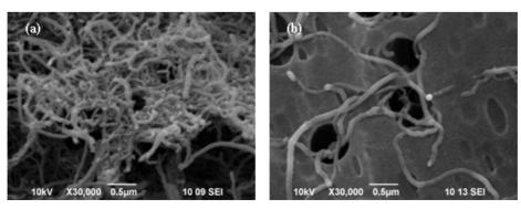
Figure 3. SEM micrographs of dispersed CNT (a) without and (b) with DI.
