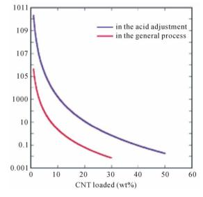
Figure 5. Electrical resistance for CNT-based paper.
