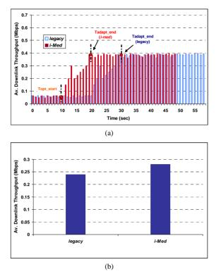
Figure 13. (a) Av. Downlink Throughput vs time; (b) Av. Downlink Throughput without (legacy) and with i-MED for Image transfer application.
