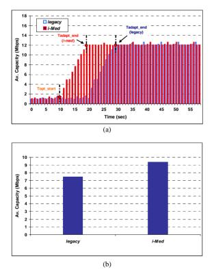
Figure 8. (a) Av. Capacity vs time; (b) Av. Capacity without (legacy) and with i-MED, for Video Conference Application.
