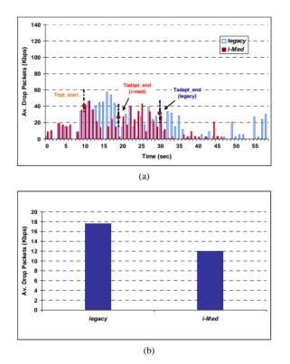
Figure 11. (a) Av. Data Dropped vs time; (b) Av. Data Dropped without (legacy) and with i-MED for Image transfer Application.
