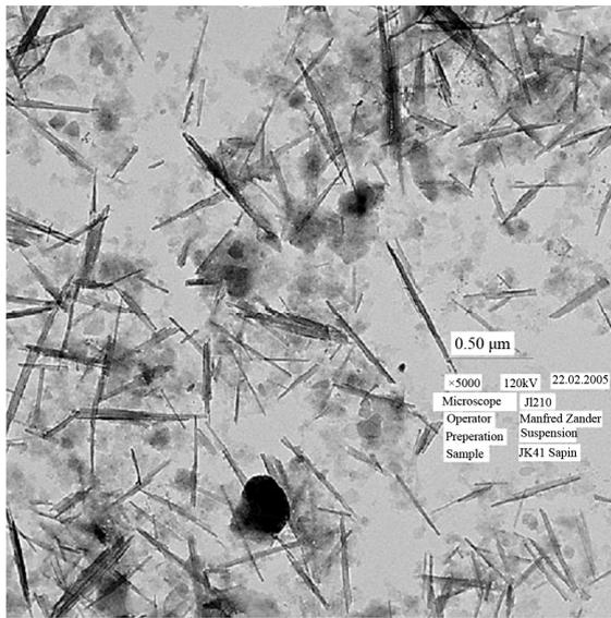
**Figure 4. Palygorskite morphology. Some montmorillonite is also present [19], (Microscopy by Zander, Greifswald University).**
