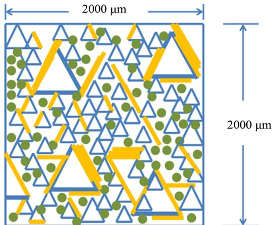
**Figure 5. Schematic view of REV of palygorskite/talc grout in 2D. It represents fine aggregate grains (blue) with cement particles (green spheres), and packets of palygorskite or talc particles appearing as thick yellow lines in the drawing. 3D equivalents were 400  $\mu\text{m}$  thick.**
