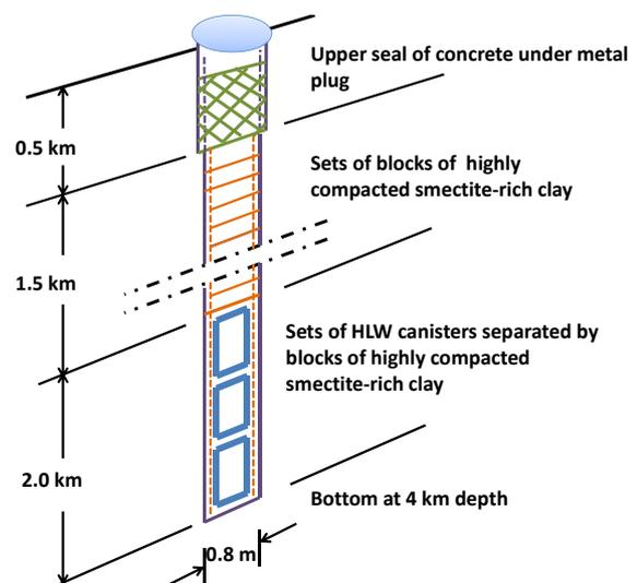
**Figure 1.** Borehole sealing by installing clay seals where the rock is tight and casting concrete where fracture zones are intersected. Left: Detail of concrete cast where the fracture zone has been sealed by grouting [12]. Right: VDH with clay seal from 0.5 to 2 km depth and with high-level radioactive waste canisters separated by clay from 2 to 4 km depth [9].
