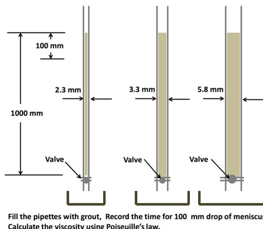
**Figure 7. Principle of grout capillary test. The pipettes are filled with grout, and the time recorded for 10 cm grout flow (subsidence of meniscus).**
