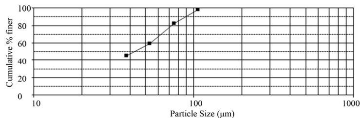
**Figure 2.** Grain size distribution of ground crushed and ground quartzite.
