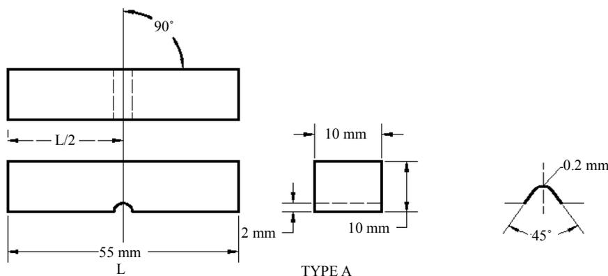
**Figure 3. Standard sample for charpy impact test.**
