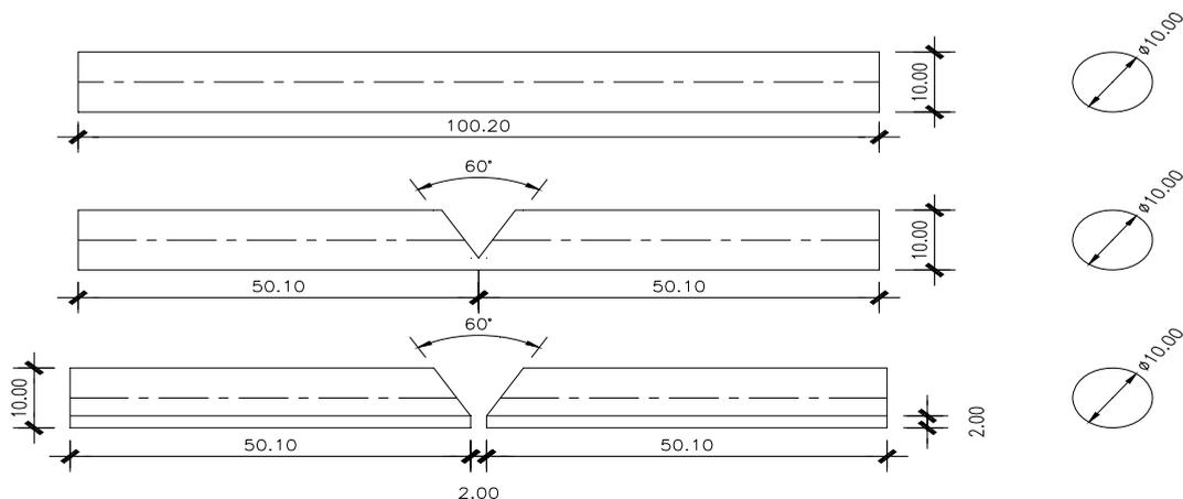
**Figure 1. Joint preparation for V-groove welding [2].**
