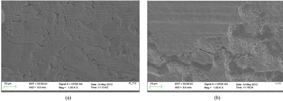
**Figure 4. (a) Micrograph of the fusion zone for sample A; (b) Micrograph of the heat affected zone for sample A.**
