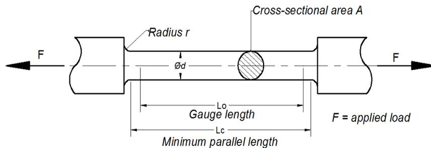
**Figure 2. Standard sample for tensile test [24]. Proportional samples (BS18) are given by the relationship.  $L_0 = 5.56\sqrt{A}$ . Since  $A = \pi d^2/4$ , then  $\sqrt{A} = d\sqrt{\pi}/2 = 0.88d$ . Thus  $L_0 = 5.65 \times 0.88 d \approx 5 d$  [24].**
