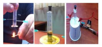
Figure 5. Plastic syringe apparatus for electrolysis designed by a participating teacher in the workshop.
