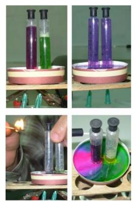
Figure 2. Plastic Syringe Huffman apparatus experiment.
