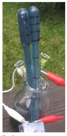
Figure 3. Two 3-ml plastic pipettes electrolysis experiment.
