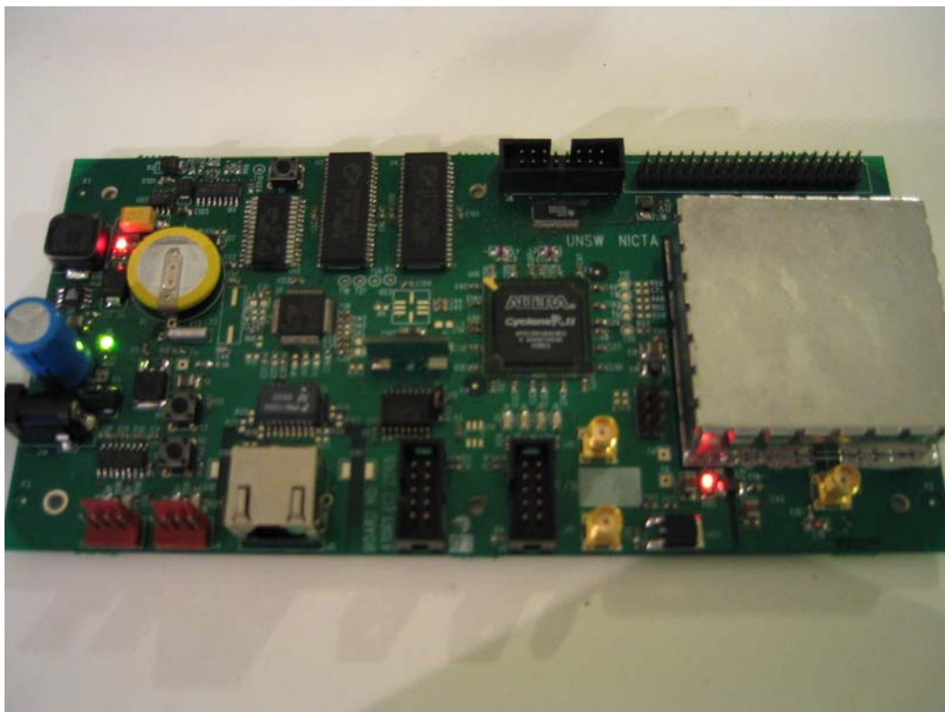
Figure 4 The new FPGA receiver board
