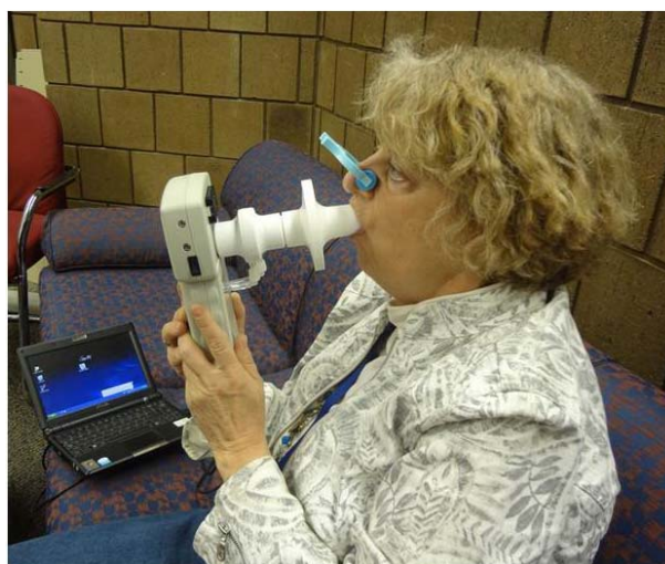
Figure 2. Subject using the hand held APD. This device was connected to a laptop computer for data recording. However, this is not required for use. All values are displayed on a screen in the field of vision.
