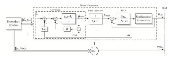
Figure 1. Diesel generator control.
