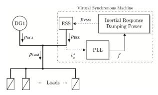
Figure 2. Diesel-based mini-grid with VSM control.
