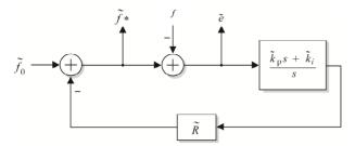
Figure 4. Open-loop estimator.
