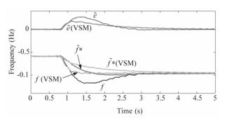
Figure 10. Load increase with gen-set operating with 6% frequency droop.
