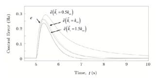
Figure 6. Influence of the integral gain  $\left( \tilde{k}_{i} \right)$  on the estimated control error.
