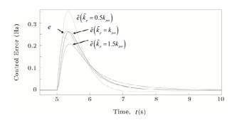
Figure 5. Influence of the proportional gain  $\left(\tilde{k}_{p}\right)$  on the estimated control error.
