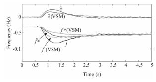
Figure 11. Load increase with gen-set operating with 3% frequency droop.
