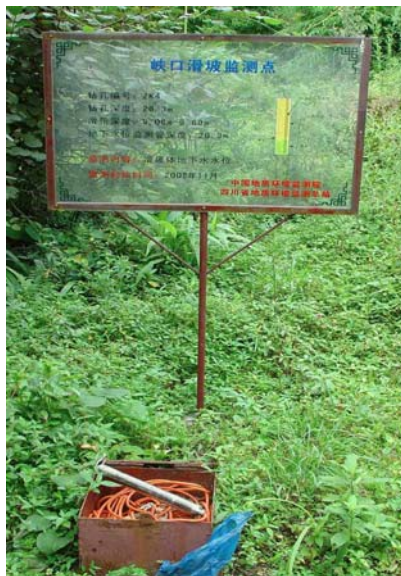
Fig. 6 Underground water level monitoring point
