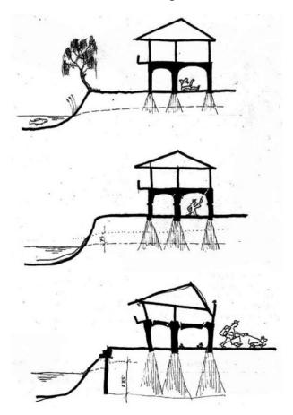
Figure 2. Changes in foundation soil caused by lowering the water level (source: Petr Pešek).
