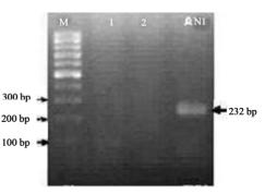
Figure 2. Detection of 232 bp amplicons of pathogenic *Aero-monas hydrophila* (AH1) on 2% agarose gel. M: Indicates the 100 bp ladder.
