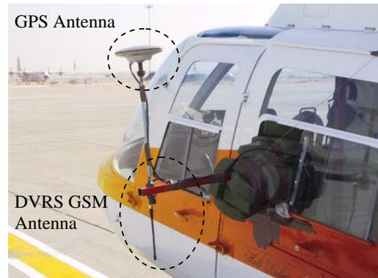
Fig. 1 System installation for the helicopter test
