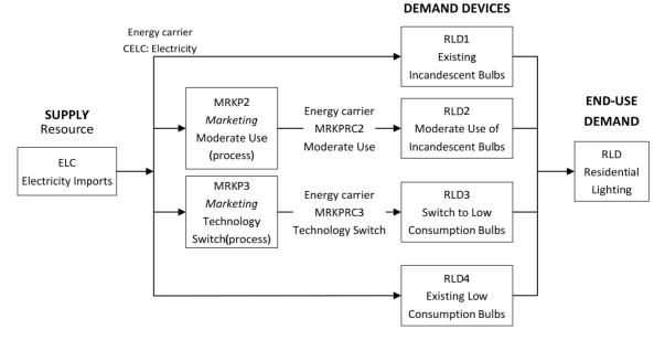
Figure 2. Structure of the reference energy system (RES).
