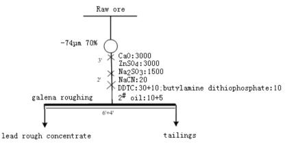
Figure 2. Flow sheet of the lead flotation circuit which use the treated wastewater, untreated wastewater and fresh water.
