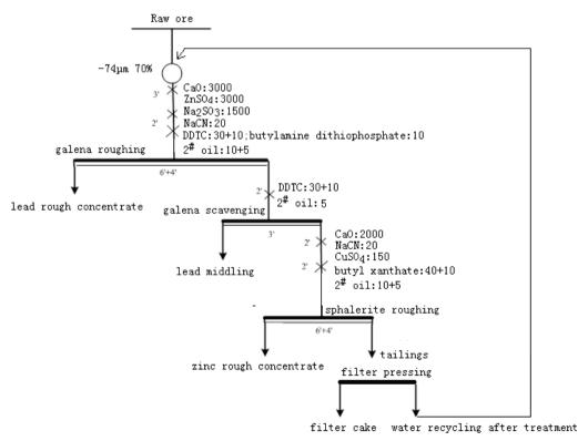
Figure 1. Flow sheet of the Zhangbeizhuan lead-zinc sulphide ore flotation process (time used were minute, concentration showed were mg/l).
