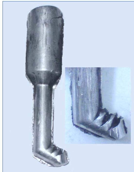
**Figure 6.** Development of cracks on the top surface of region (E) of Ex-ECAPed samples.
