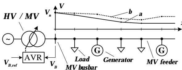
**Figure 1.** Voltage profiles in a MV feeder with and without Distributed Generators
