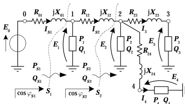
Figure 4. The per-phase equivalent circuit
