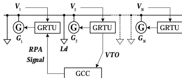
**Figure 2.** Voltage control using GRTU and GCC
