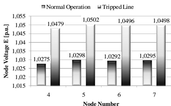
**Figure 6.** Load-Flow results with the Network Normal Operation
