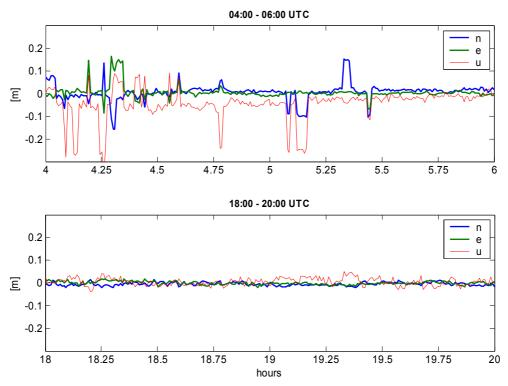
Fig. 11 Instantaneous RTK position residuals with respect to the known coordinates; 2-hour windows, KNTN-DEFI (~100 km); 1 cm constraint (1 sigma) for the ionospheric correction was applied to the "best" window (bottom) and 5 cm for the "worst" window (top).
