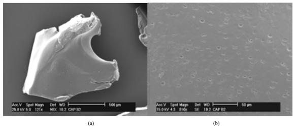
Figure 5. (a) SEM analysis showing a particle of CAPB. (b) A detail of Figure 5(a).
