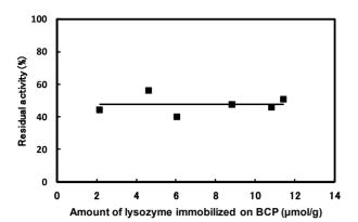
Figure 9. The effect of the amount of lysozyme immobilized on the residual activity of immobilized lysozyme after the heat treatment at 90°C for 30 min.
