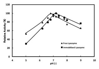
Figure 5. The effect of pH on the activity of free and immobilized lysozyme at 25°C. The relative activity at optimum pH is taken as 100%.
