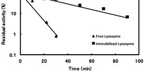
Figure 8. Time course of residual activity of free and immobilized lysozyme through the heat treatment at pH 7.0 and 90°C.
