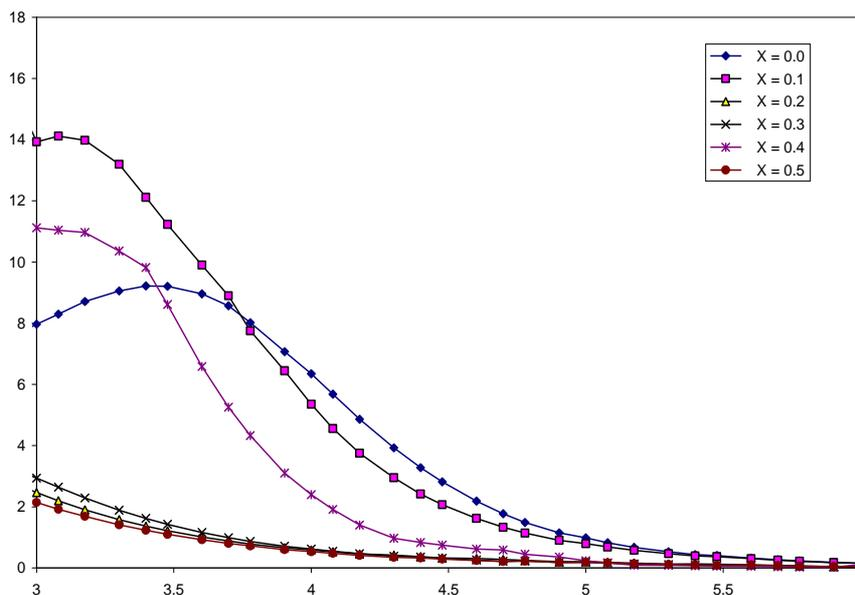
Figure 7. The plot of dielectric loss tangent ( $\tan\delta$ ) vs  $\log f$  for ferrite system  $\text{Li}_{0.35}\text{Cd}_x\text{Ti}_x\text{Mn}_{0.1}\text{Fe}_{2.55-2x}\text{O}_4$ .
