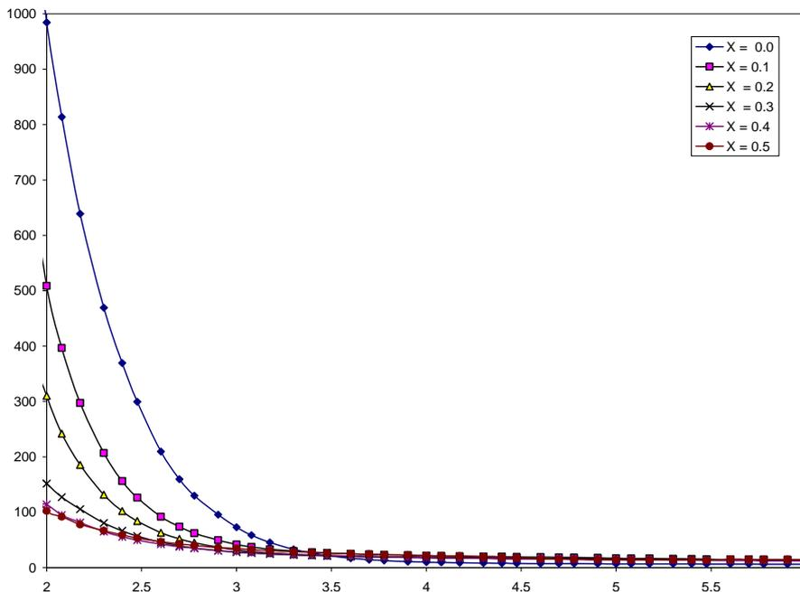
Figure 6. Variation of dielectric constant  $\epsilon'$  vs  $\log f$  for ferrite system  $\text{Li}_{0.35}\text{Cd}_x\text{Ti}_x\text{Mn}_{0.1}\text{Fe}_{2.55-2x}\text{O}_4$ .
