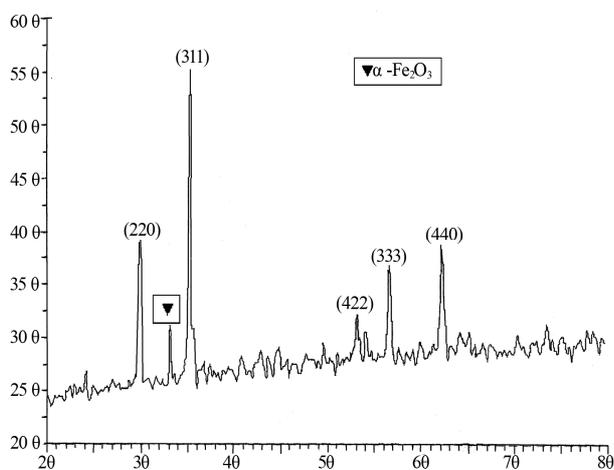
**Figure 1.**  $\text{Fe}_2\text{O}_3$  pattern XRD of  $\text{Li}_{0.35}\text{Cd}_{0.3}\text{Ti}_{0.3}\text{Mn}_{0.1}\text{Fe}_{1.95}\text{O}_4$ .
