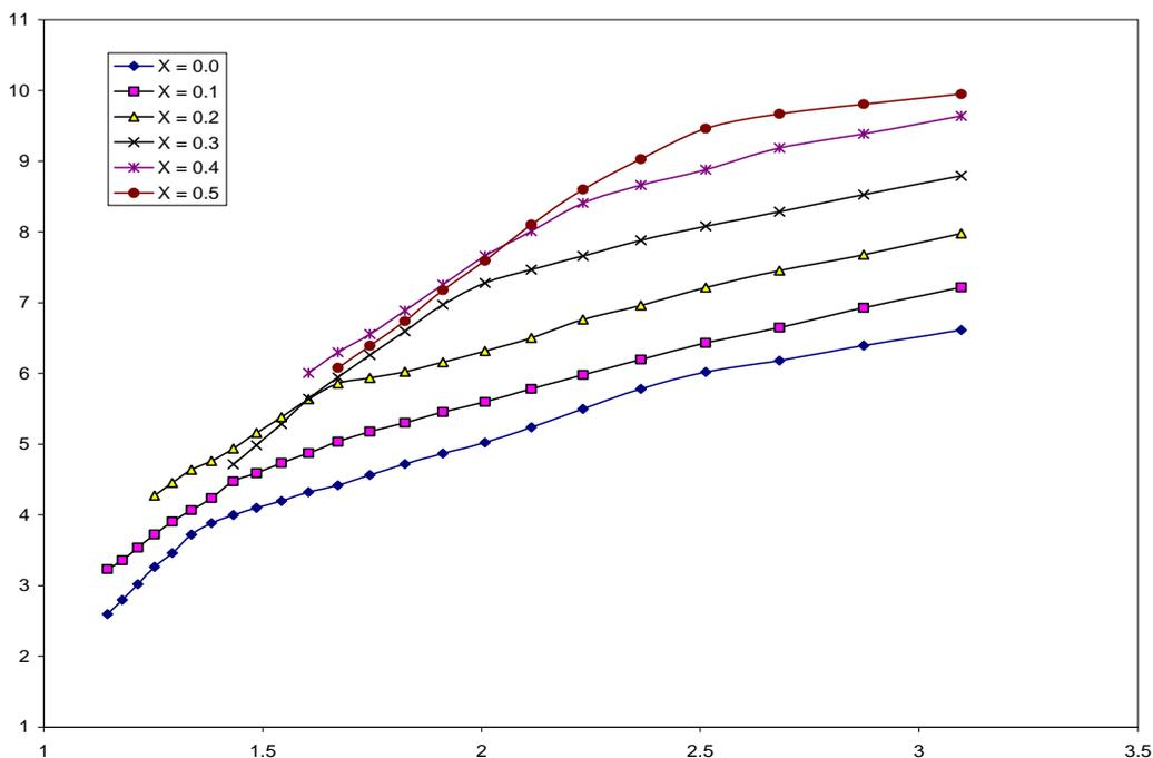
Figure 5. Variation of  $\log \rho$  vs  $10^3/T$  for  $\text{Li}_{0.35}\text{Cd}_x\text{Ti}_x\text{Mn}_{0.1}\text{Fe}_{2.55-2x}\text{O}_4$ .
