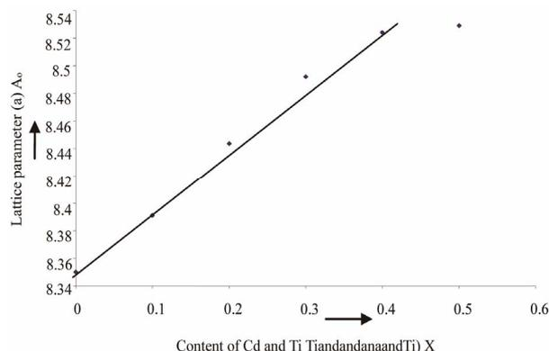
**Figure 2.** Variation of lattice parameter with Cd and Ti content [x] in  $\text{Li}_{0.35}\text{Cd}_x\text{Ti}_x\text{Mn}_{0.1}\text{Fe}_{2.55-2x}\text{O}_4$  series.
