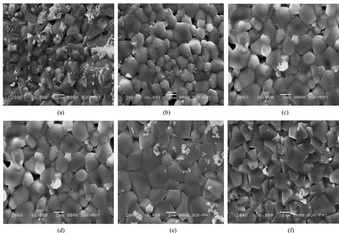
**Figure 3.** SEM of series  $\text{Li}_{0.35}\text{Cd}_x\text{Ti}_x\text{Mn}_{0.1}\text{Fe}_{2.55-2x}\text{O}_4$  with  $x = 0$  to  $0.5$ .
