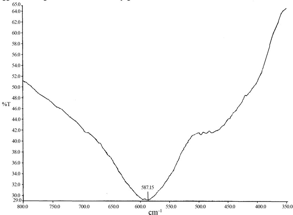
Figure 4. IR spectra of  $\text{Li}_{0.35}\text{Cd}_x\text{Ti}_x\text{Mn}_{0.1}\text{Fe}_{2.55-2x}\text{O}_4$  with  $x = 0.3$ .
