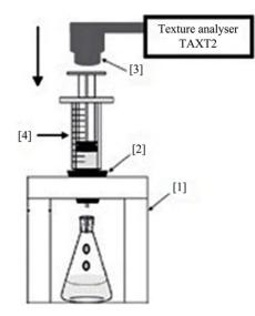
Figure 1. Experimental set-up for the measurement of the syringeability force developed during injection: 1) metallic support; 2) plastic clamping ring; 3) force transducer and 4) syringe (adapted from reference [22]).
