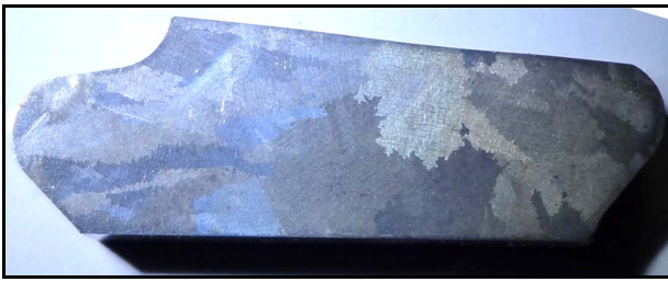
Figure 1. Sectioned and macro-etched specimen (5 \times ).
