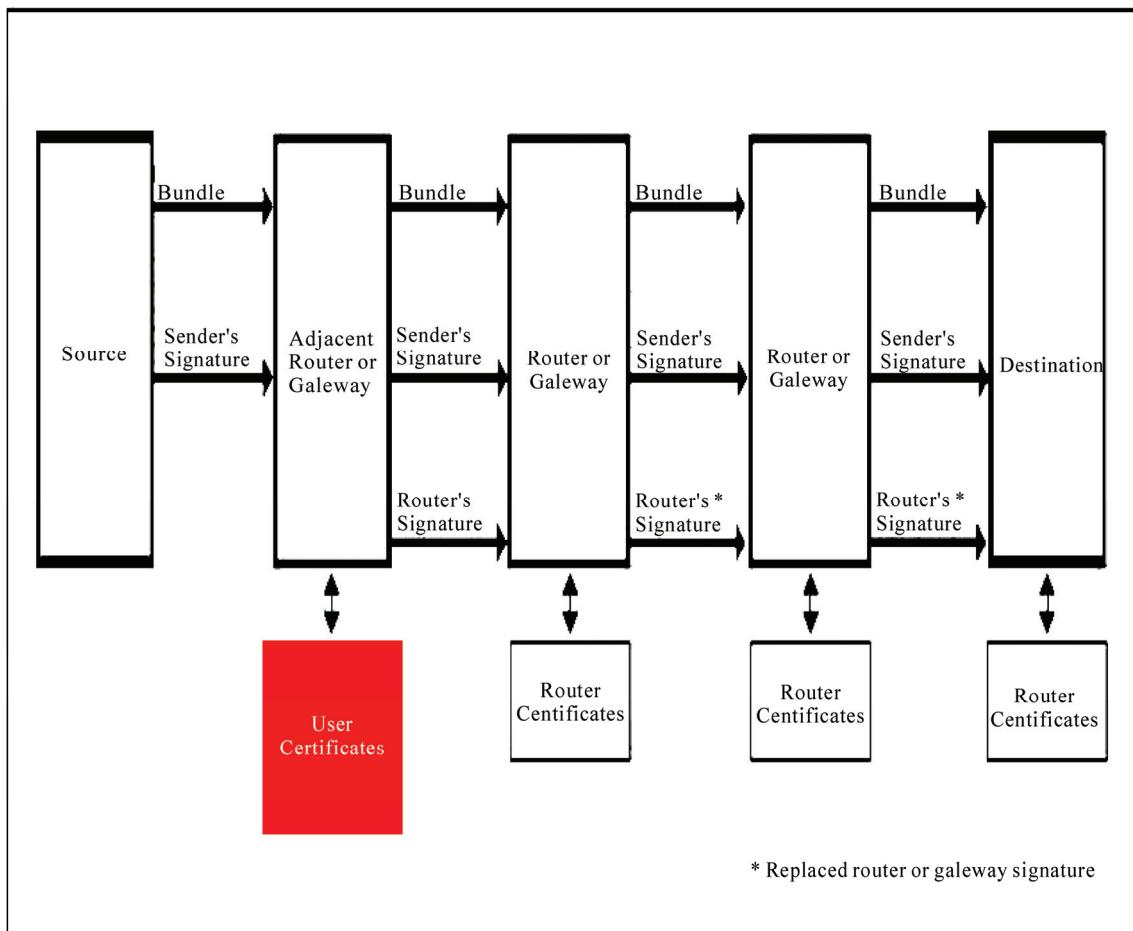
**Figure 1. Security steps using public key cryptography [9].**
