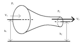
**Figure 1.** Model of fluid dynamics in lumen. V: Flow rate, P: pressure, h: height.
