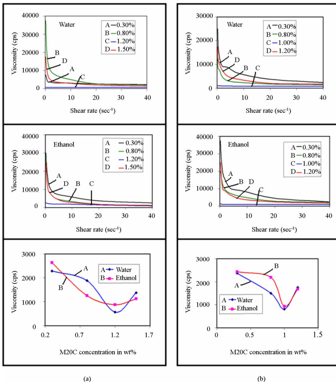
**Figure 6.** Plots of viscosity against shear rate for different concentration of M20C deflocculant (dispersant) in water and ethanol system and plots of viscosity against M20C concentration (at constant shear rate of 40 sec<sup>-1</sup>). (a) ZrO<sub>2</sub> (b) 12 Ce-TZP powders.
