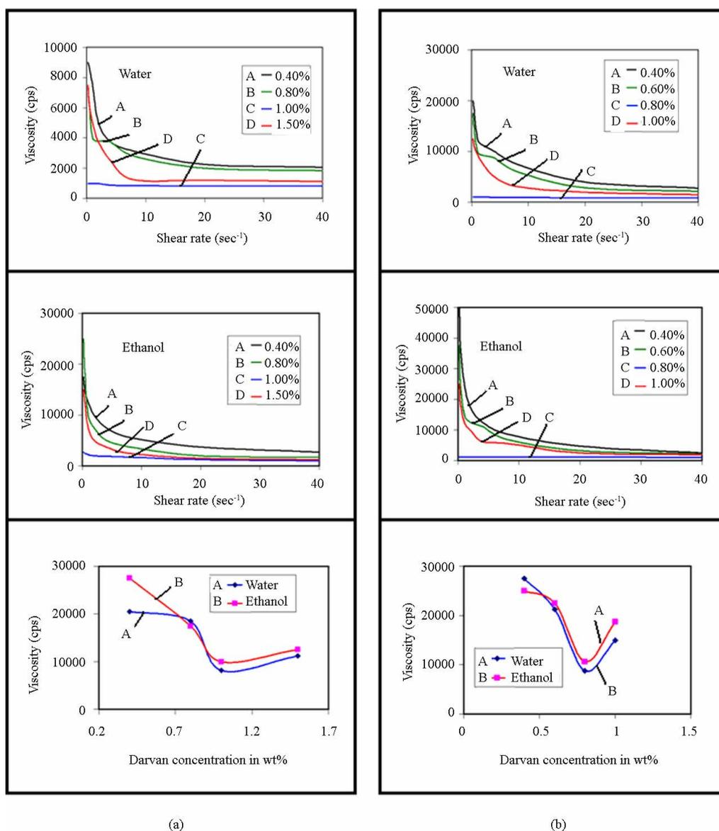
**Figure 5.** Plots of viscosity against shear rate for different concentration of Darvan deflocculant (dispersant) in water and ethanol system and plots of viscosity against Darvan concentration (at constant shear rate of 40 sec<sup>-1</sup>). (a)  $ZrO_2$ ; (b) 12 Ce-TZP powders.
