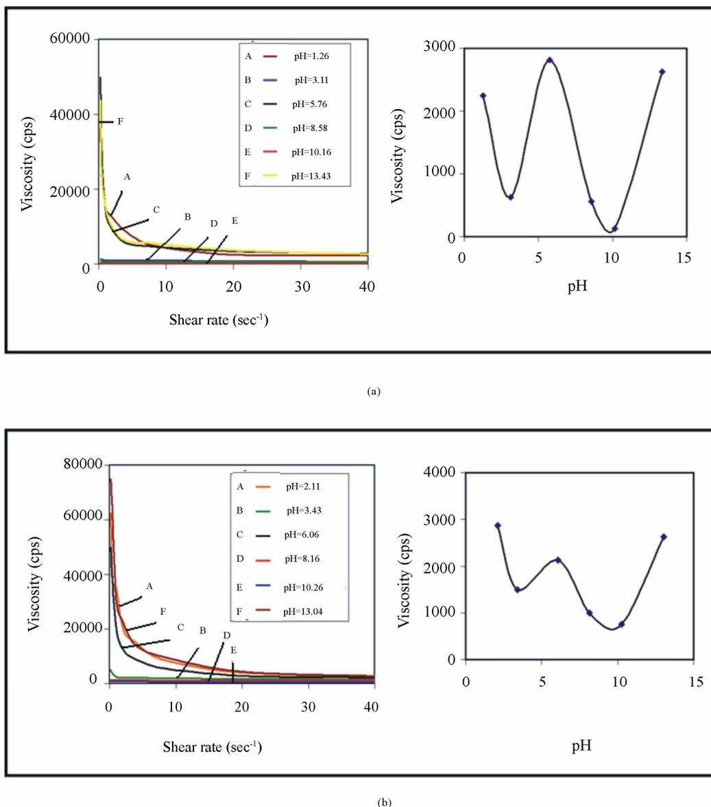
**Figure 7.** Plots of viscosity against shear rate for suspensions with pH values indicated and plots of viscosity against several pH values (at constant shear rate of  $40 \text{ sec}^{-1}$ ). (a) 80 wt.% zirconia-20 wt.% water-M20C deflocculant; (b) 75 wt.% 12 Ce-TZP-25 wt.% water-M20C deflocculant.
