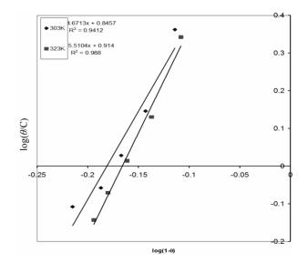
Figure 4. Flory-Huggins isotherm for adsorption of ethanol extract of *Vernonia amgydalina* on the mild steel surface.
