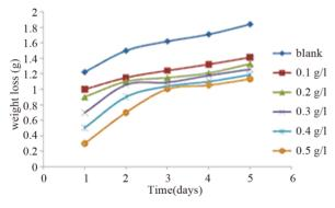
Figure 1. Variation of weight loss with different concentrations of *Vernonia amygdalina* extract for the corrosion of mild steel in 0.2 M H<sub>2</sub>SO<sub>4</sub> at 303 K.
