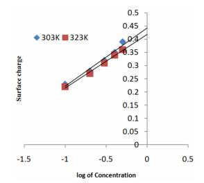
Figure 3. Temkin isotherm for adsorption of ethanol extract of *Vernonia amygdalina* on the surface of mild steel.
