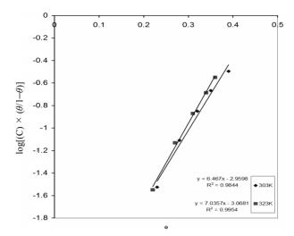
Figure 5. Frumkin isotherm for adsorption of ethanol extract of *Vernonia amgydalina* on the mild steel surface.
