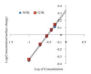
Figure 2. Langmuir isotherm for adsorption of ethanol extract of *Vernonia amygdalina* on mild steel surface.
