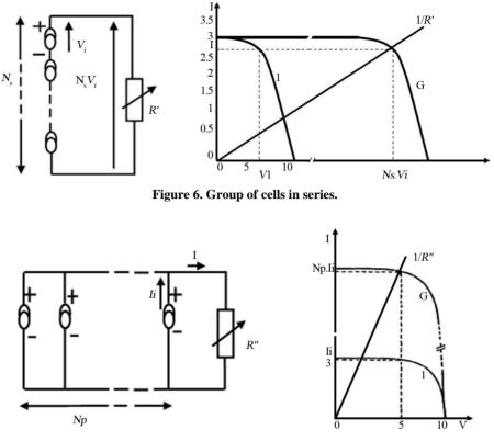
Figure 7. Group of cells in parallel [11].
