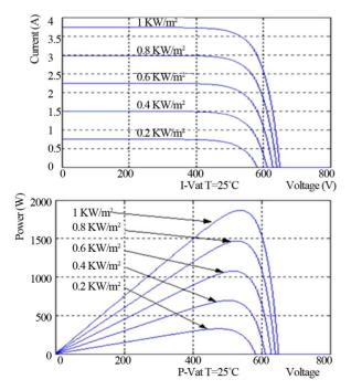
Figure 4. Influence of the illumination at  $T = 25^{\circ}$ C.
