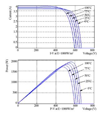
Figure 5. Influence of temperature for a light, E = 1000 W/m<sup>2</sup>.
