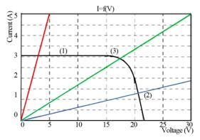
Figure 3. Current-voltage characteristics of photovoltaic modules  $E = 1000 \text{ W/m}^2$ ,  $T = 25^{\circ}\text{C}$ .
