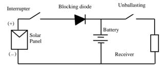
Figure 10. Diagram of a control series.
