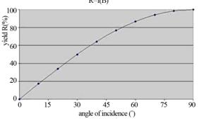
Figure 8. Graph representing the performance against the angle of incidence.
