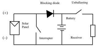
Figure 11. Diagram of a shunt regulator [12].
