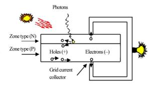
Figure 1. Principle of operation of a photovoltaic cell.
