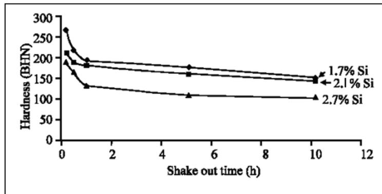
Fig.3:Plot of effect of shake-out time on hardness
