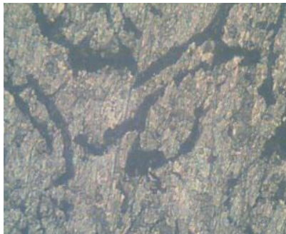
(a) Unalloyed, annealed at 800°C
