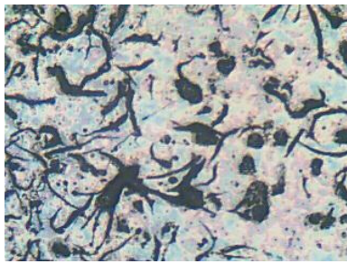
(a) Unalloyed, normalized at 800°C
