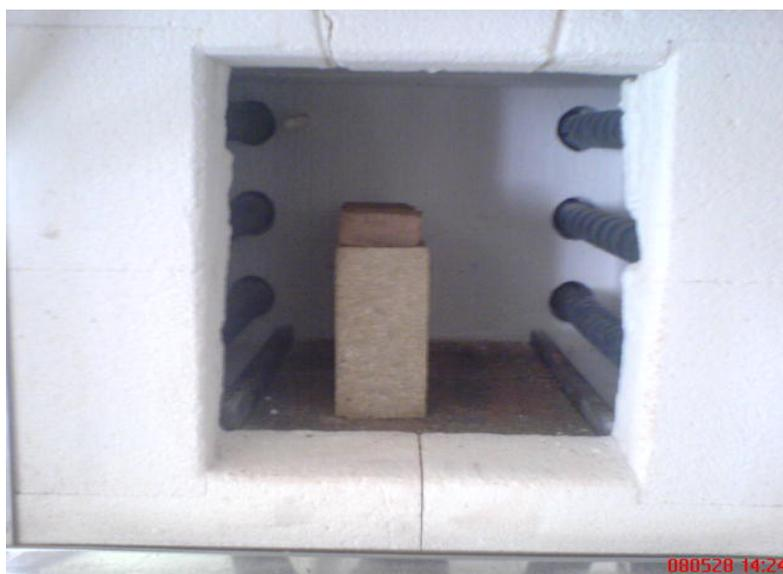
Plate 1. The Samples placed inside the furnace for firing
