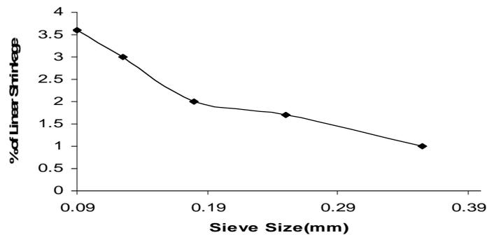
Figure 3. Variation of Linear Shrinkage with Sieve Size.
