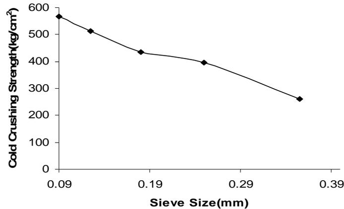
Figure 4. Variation of Cold Crushing Strength with Sieve Size.
