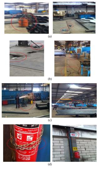
Figure 10. (a) Negligence in storage materials and tools; (b) Negligence in providing and maintaining the facilities & utilities; (c) Negligence of worker; (d) Negligence of management in displaying the safety rules.
