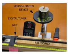
Figure 2. A detail of our experimental apparatus, showing the spring-loaded device pressing at the fifth fret position. The resulting string deformation and the slight change in the string tension will cause the lack in intonation of the note being produced. The digital tuner positioned near the sonometer can accurately measure the sound frequency.
