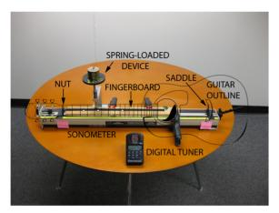
Figure 1. Our tabletop apparatus composed of a sonometer and a guitar fingerboard, with twenty metallic frets. Also shown are the two movable bridges, which simulate the nut and saddle of a guitar, the spring-loaded device used to press on the string at different positions, and the digital tuner used to measure sound frequencies. A guitar outline is superimposed on the picture, in order to show how the apparatus simulates the functionality of a real guitar.
